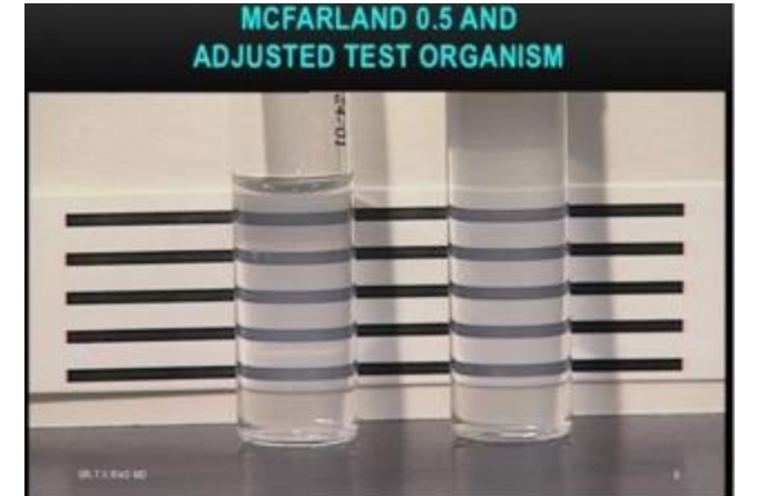
Bacterial suspension prepared to match the turbidity of the 0.5 McFarland turbidity standard
