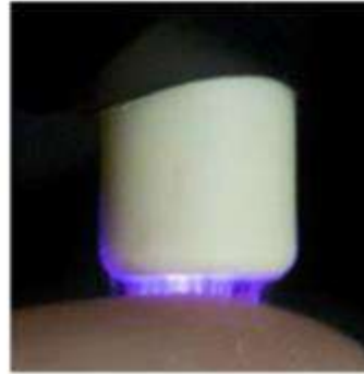
Volume dielectric barrier discharge (DBD)
