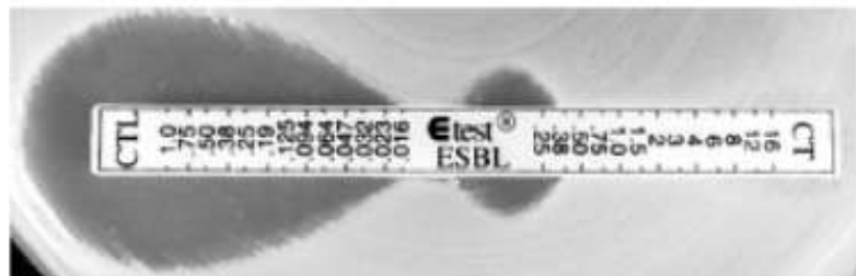
Figure 5. A "rounded" phantom inhibition zone below CT indicative of ESBL.
