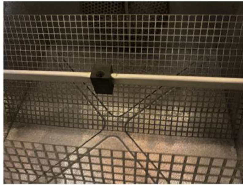
Figure 5. Grids between the air ducts and the air outlets.
