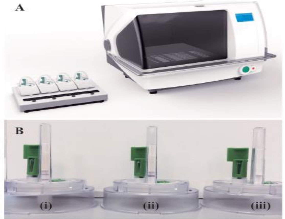
FIG 1 SAMBA semi-Q system. (A) SAMBAprep (right) and SAMBAamp (left) instruments. (B) SAMBAamp cartridge showing results for (i) >1,000 and (ii) <1,000 copies/ml and (iii) invalid results.
